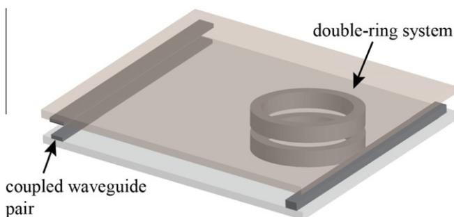
Fig. 8. Schematic design of a self-tuning resonator, adapted from Ref. [28].
