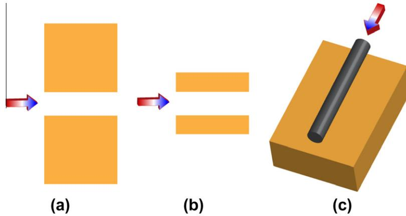
**Fig. 6.** Optical forces generated in plasmonic devices: (a) semi-infinite metal plates separated by an air gap, (b) finite-thickness metal waveguides separated by an air gap, and (c) a hybrid plasmonic system with a dielectric waveguide and a metallic substrate.
