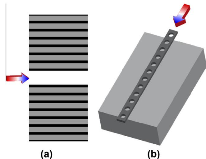
**Fig. 5.** Devices that enhance optomechanical effects via slow light: (a) waveguide formed by reflective multilayer films, (b) one-dimensionally periodic photonic crystal waveguide coupled with silica substrate.
