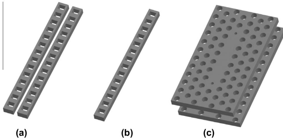
**Fig. 3.** Schematic of photonic crystal cavities showing opto-mechanical coupling. (a) “zipper” cavity, (b) nanobeam cavity, and (c) double-layer photonic crystal slab cavities. In (a) and (b), the lattice constant near the center of the device is decreased slightly (not shown) to form a microcavity.
