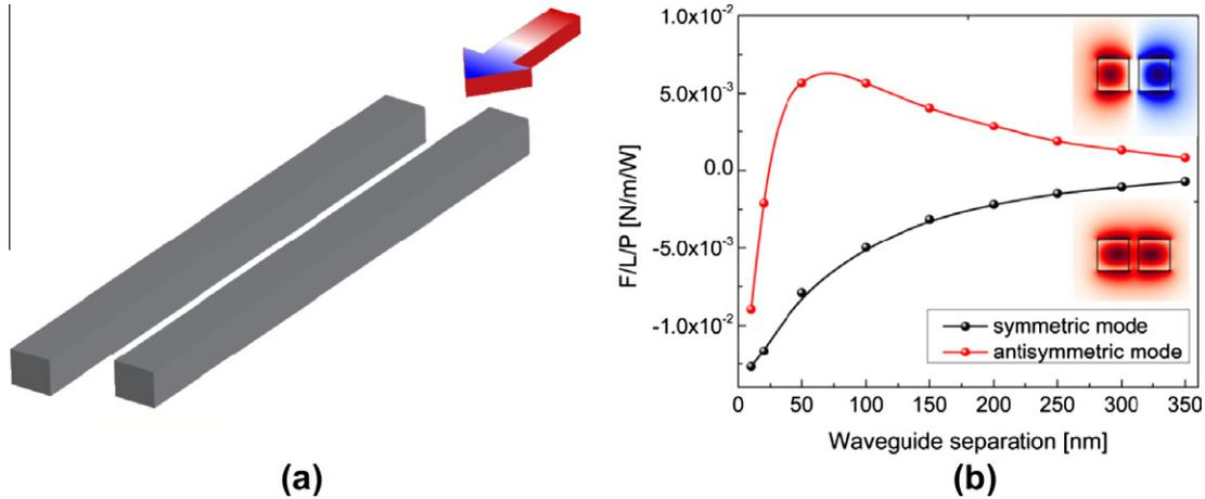
**Fig. 1.** Optical forces between parallel waveguides. (a) Schematic structure; multicolored arrow indicates the direction of light propagation. (b) Calculated, normalized, optical force as a function of waveguide separation. Insets show modal profiles, with red/blue indicating positive/negative values of the electric field component parallel to the air gap.
