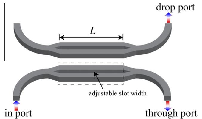
**Fig. 7.** Optically-tunable directional coupler, in which the effective index of each arm is tuned via an adjustable slot width. Figure adapted from [70].
