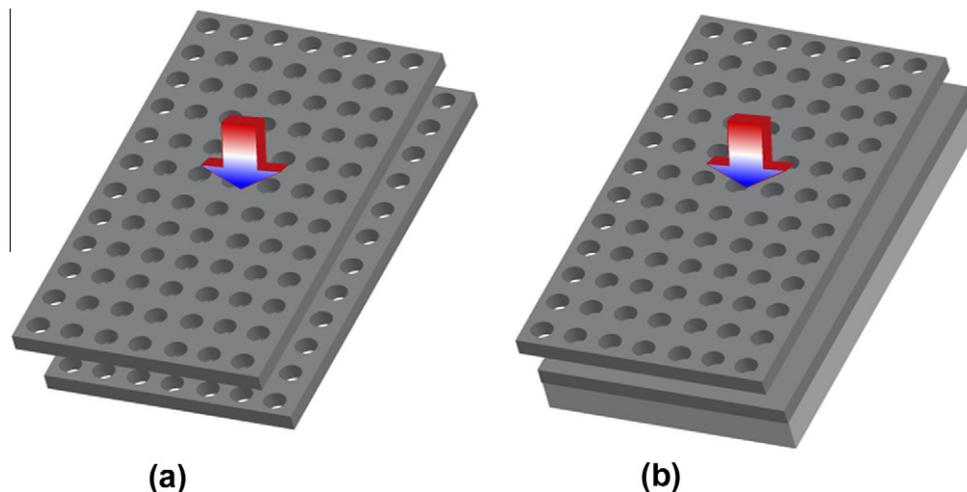
**Fig. 4.** Guided-resonance optomechanical devices: (a) double-layer photonic crystal slab supporting guided resonances, and (b) asymmetric guided resonant structure composed of photonic crystal slab and silicon-silica substrate.
