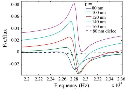
Fig. 2. (Color online) Vertical force on gold nanoparticles of different sizes and a dielectric particle with  $r = 80$  nm and  $\epsilon = 1.59$ .
