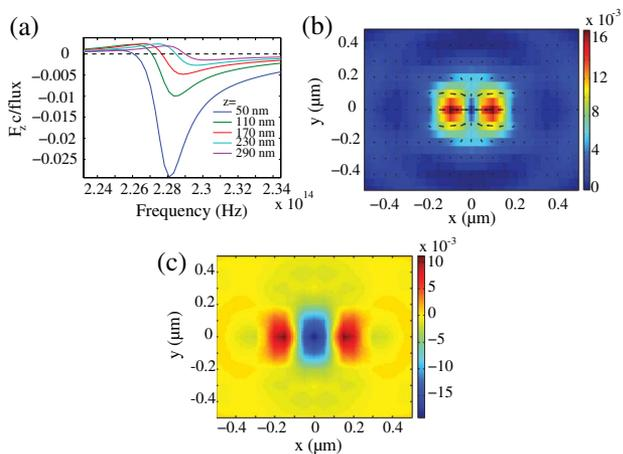
Fig. 3. (Color online) (a) Vertical force as a function of frequency for several different vertical positions. Normalized force in the (b) horizontal and (c) vertical directions as a function of position in the  $x$ - $y$  plane for a gold particle with  $r = 80$  nm.
