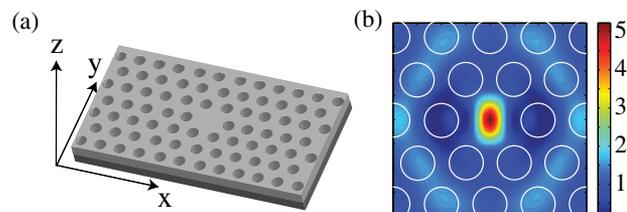
Fig. 1. (Color online) (a) Photonic crystal microcavity. (b) Electric field intensity above the slab slightly off resonance.
