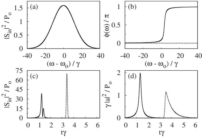
FIG. 2. (a) The power spectrum of an input pulse. (b) Phase spectra of the transform-limited pulse (dotted line) and a shaped pulse [Eq. (3)] (solid line). (c) Shaped pulse (solid line) and transform-limited pulse (dotted line) in the time domain, with power and phase spectra shown in Figs. 2(a) and 2(b), respectively. (d) Reflected power from the resonator [ $|a(t)|^2$  is the energy coupled into the resonator].
