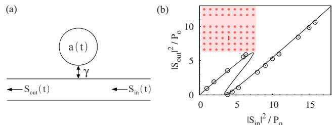
FIG. 1. (Color online) (a) Schematic of a coupled resonator-waveguide system.  $a(t)$  is the modal amplitude of the resonator,  $\gamma$  is its coupling rate to the waveguide, and  $S_{\text{in}}(t)$  [ $S_{\text{out}}(t)$ ] is the incoming [outgoing] wave in the waveguide. (b) Input vs output power plot obtained from CMT (solid line) and FDTD (open circles) for the coupled resonator-waveguide PC device shown in the inset.
